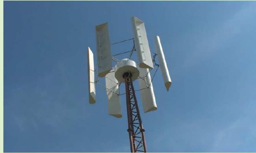
Freewindenergy vertical axis wind generator
