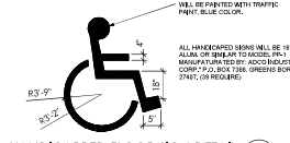
HANDICAPPED FLOOR SIGN DETAIL NOT TO SCALE
