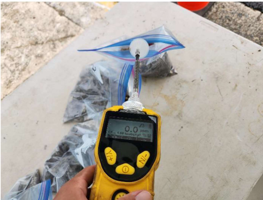
Photograph 22: PID screening in soil sample SB-1. PID = 0.0 ppm.
