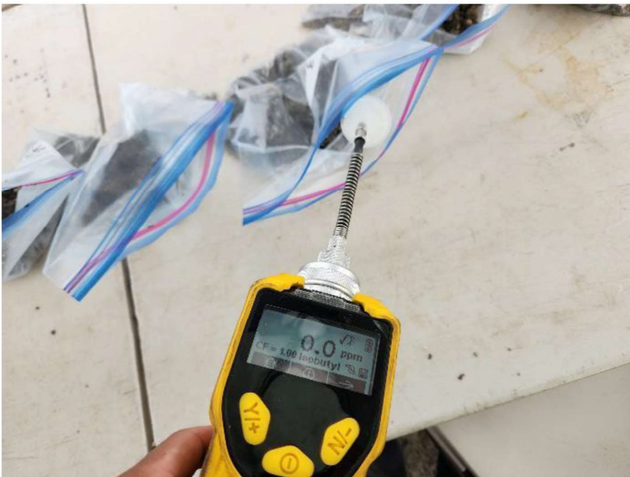
Photograph 24: PID screening in soil sample SB-3. PID = 0.0 ppm.
