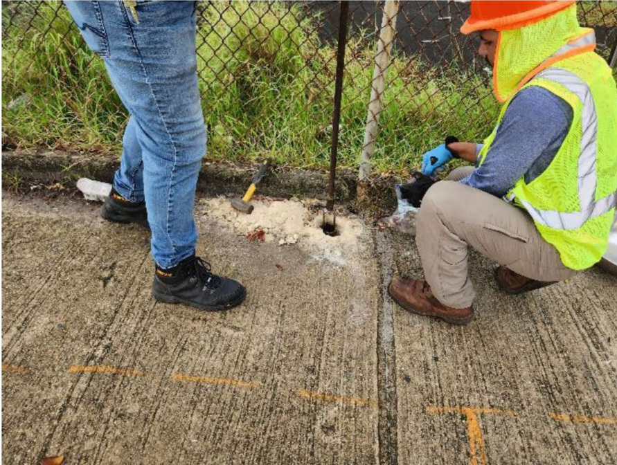
Photograph 5: Soil drilling using a hand auger at SB-1.
