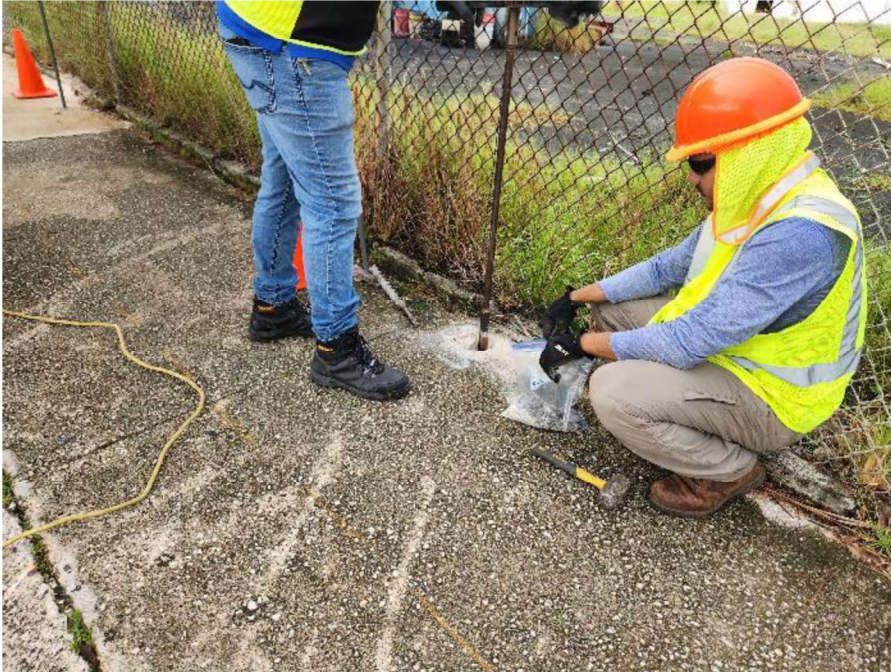
Photograph 11: Soil drilling using a hand auger at SB-3.
