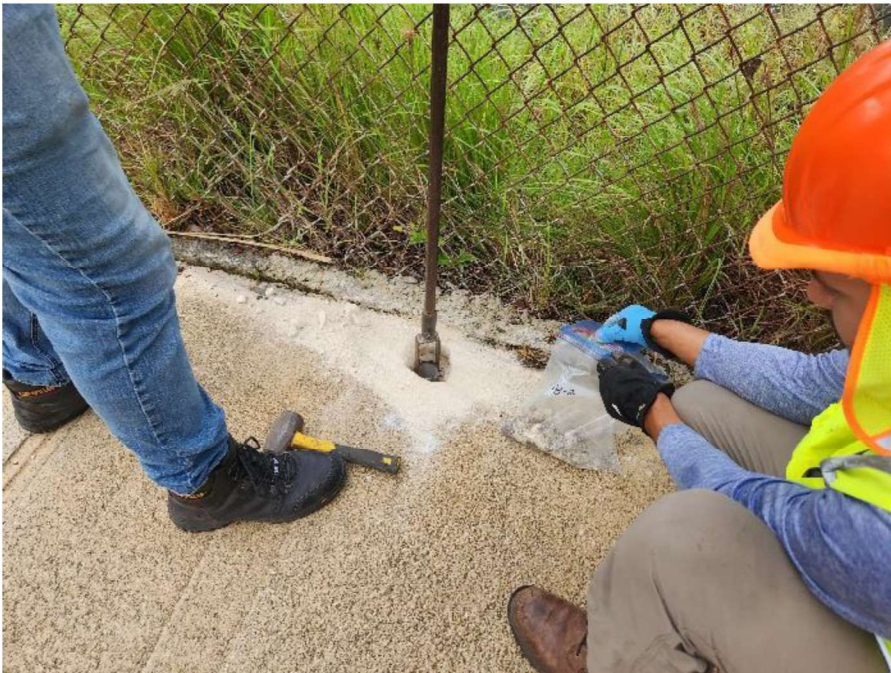
Photograph 8: Soil drilling using a hand auger at SB-2.
