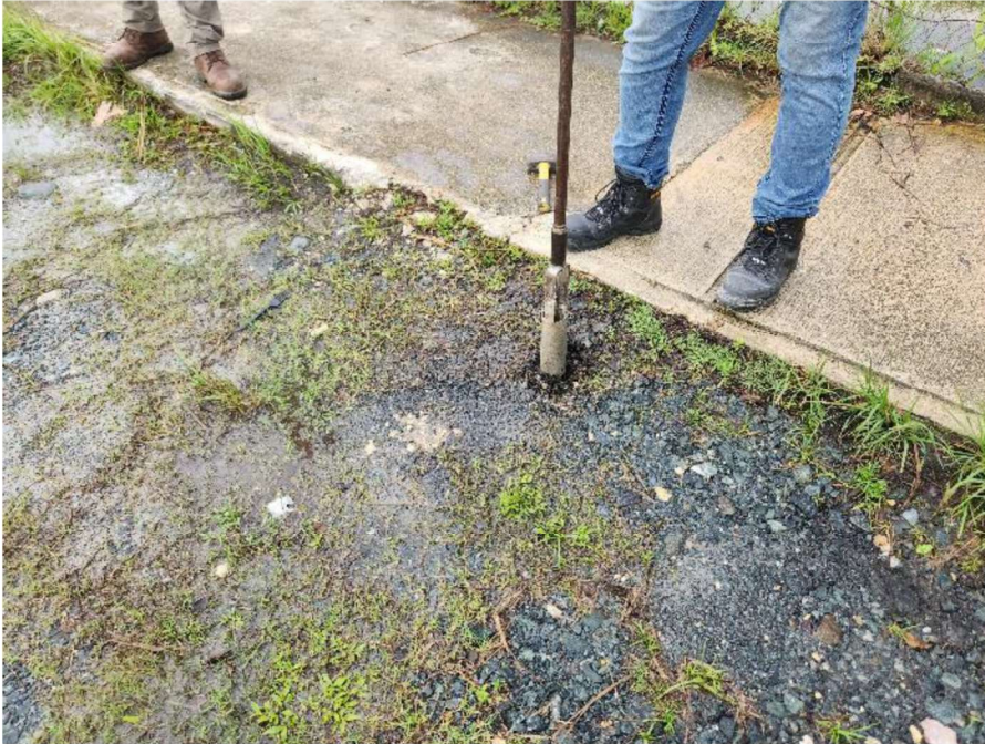
Photograph 19: Soil drilling using a hand auger at SB-6.
