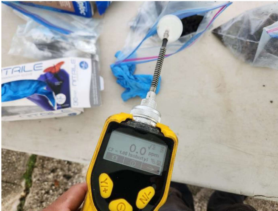
Photograph 27: PID screening in soil sample SB-6. PID = 0.0 ppm.
