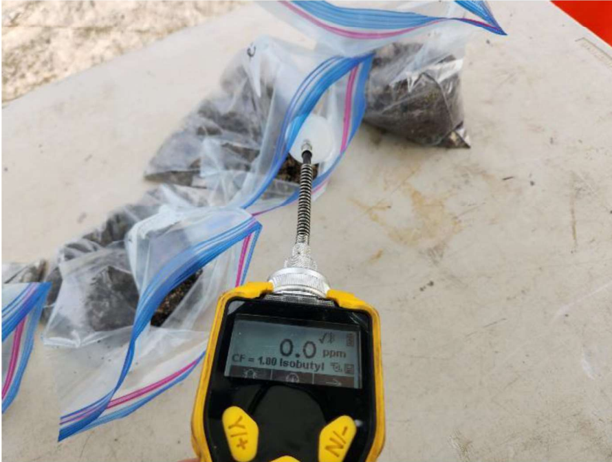
Photograph 23: PID screening in soil sample SB-2. PID = 0.0 ppm.
