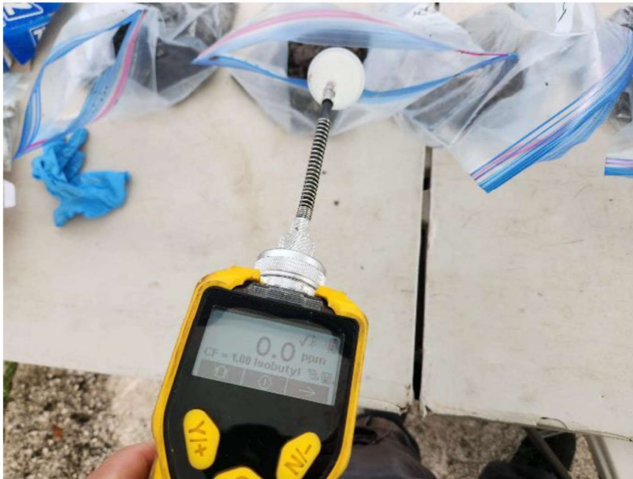
Photograph 26: PID screening in soil sample SB-5. PID = 0.0 ppm.
