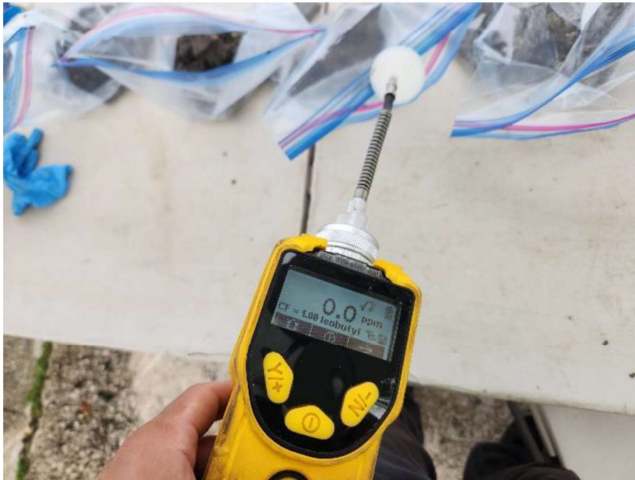
Photograph 25: PID screening in soil sample SB-4. PID = 0.0 ppm.
