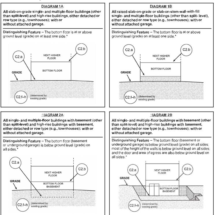
\* A floor that is below ground level (grade) on all sides is considered a basement even if the floor is used for living purposes, or as an office, garage, workshop, etc.
