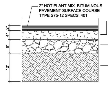
CRUSHED STONE CLASS "I" GRADATION "A" MAX. 0.0381 (SPECS 304 & 401)
