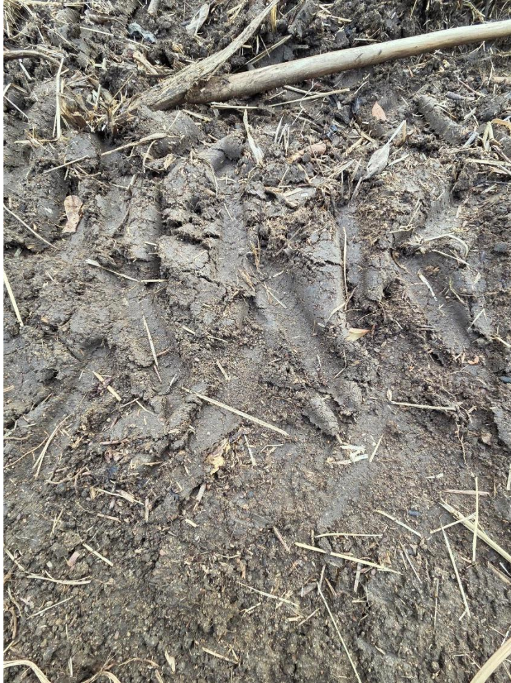
Photo 5 -The soil at the project site shows a clayey composition with poor to moderate drainage, consistent with NRCS classifications for Yabucoa. Based on field observations, it resembles Parcelas clay or Coloso clay, which are not classified as hydric soils under NRCS criteria
