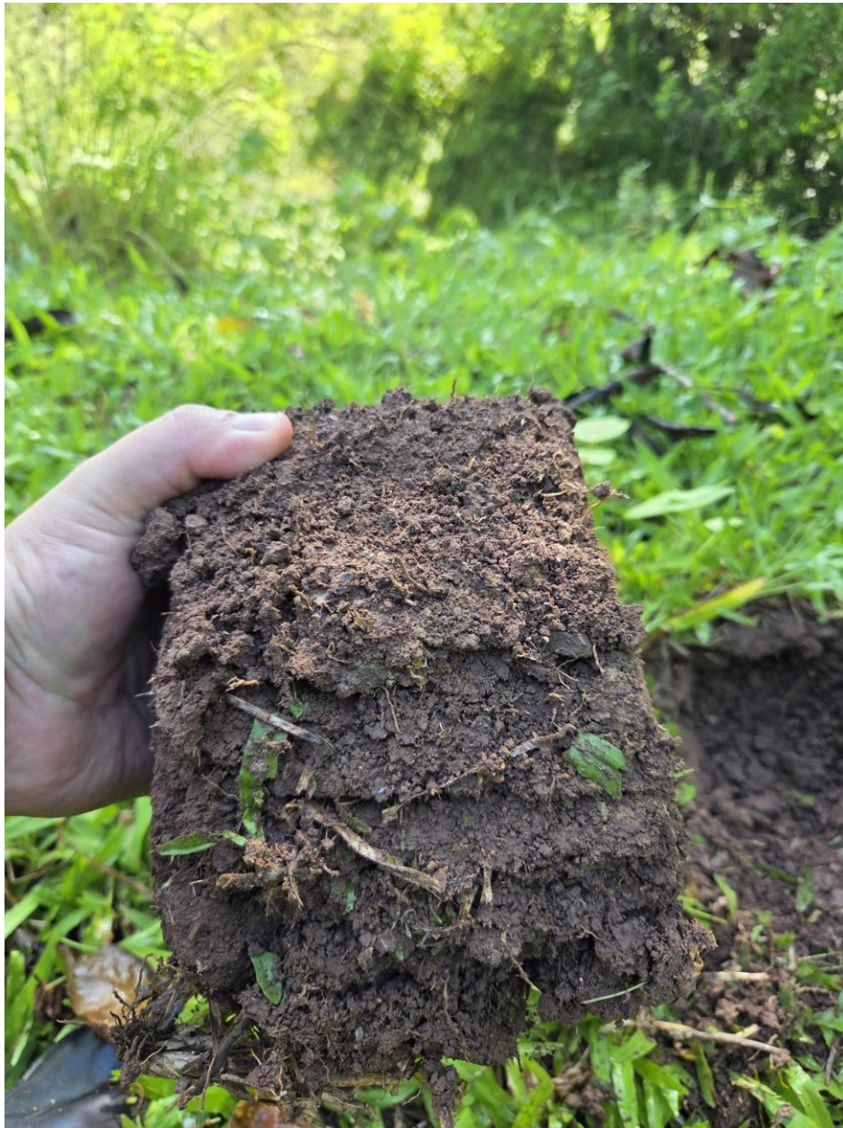
Photo 3 - Soil profile extracted from the Ciales project site showing brown clay with root fragments and organic matter near the surface. The structure and texture are consistent with USDA-NRCS mapped soils in the area (Humatas, Morado, and Mucara series) on steep slopes. The profile indicates well-drained conditions without evidence of hydric characteristics
