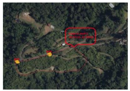
The Scope of Work 3 is the construction of a fence, with wood posts of 6' long and metal wire, of approximately 2,200 feet located at 18.27234, -67.05709. The maximum expected ground disturbance is 3 feet. This area will have two gates, as shown below.
