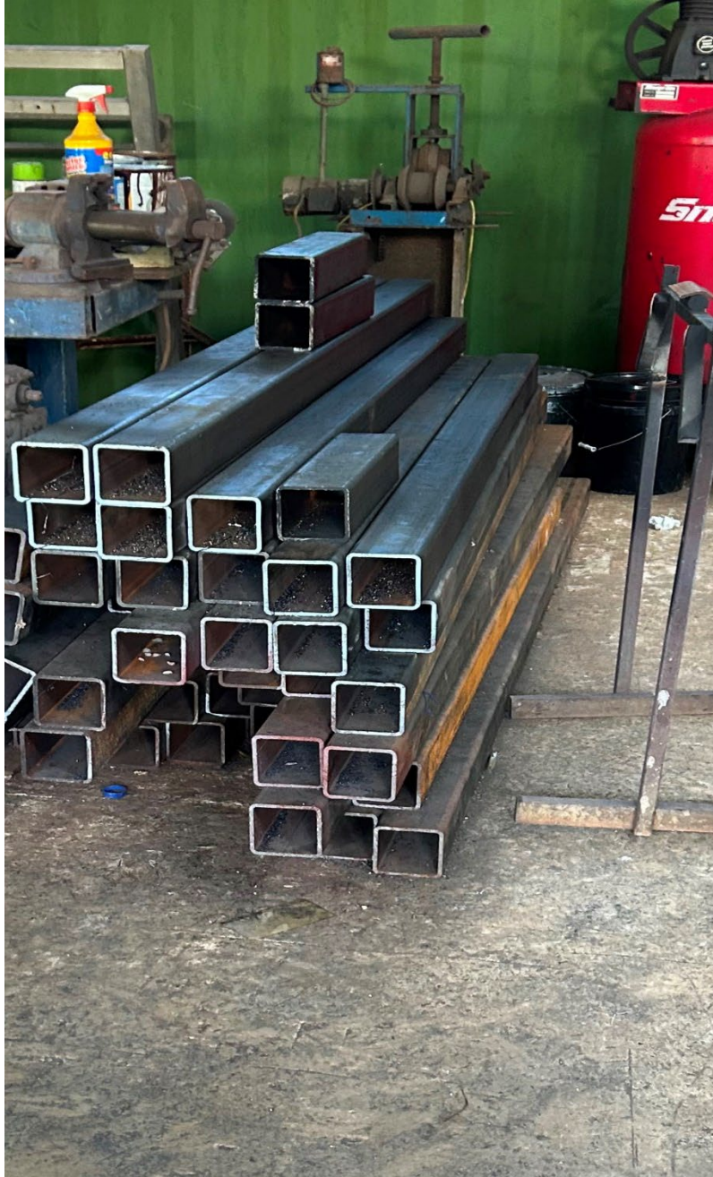
Materials for base of generator when installed.
