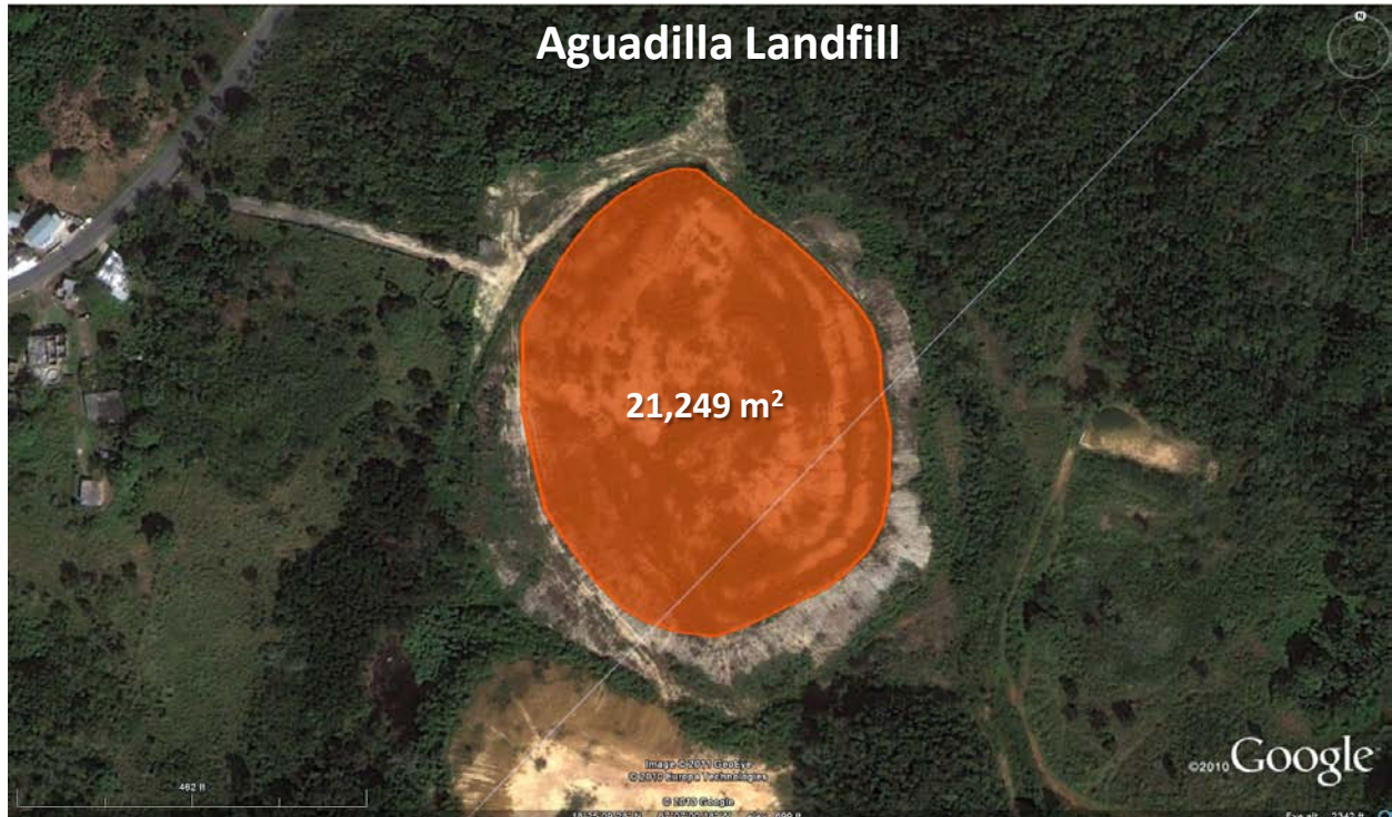
Figure 6. Aerial view of the feasible area for PV at the Aguadilla Landfill
