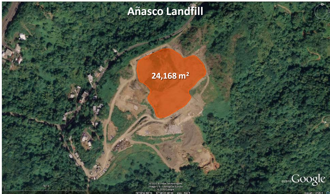
Figure 8. Aerial view of the feasible area for PV at the Añasco Landfill
