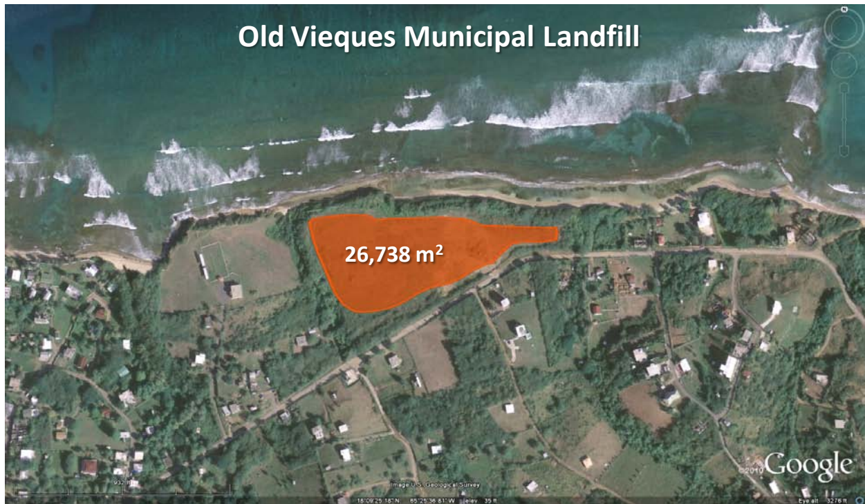
Figure 31. Aerial view of the feasible area for PV at the Old Vieques Municipal Landfill
