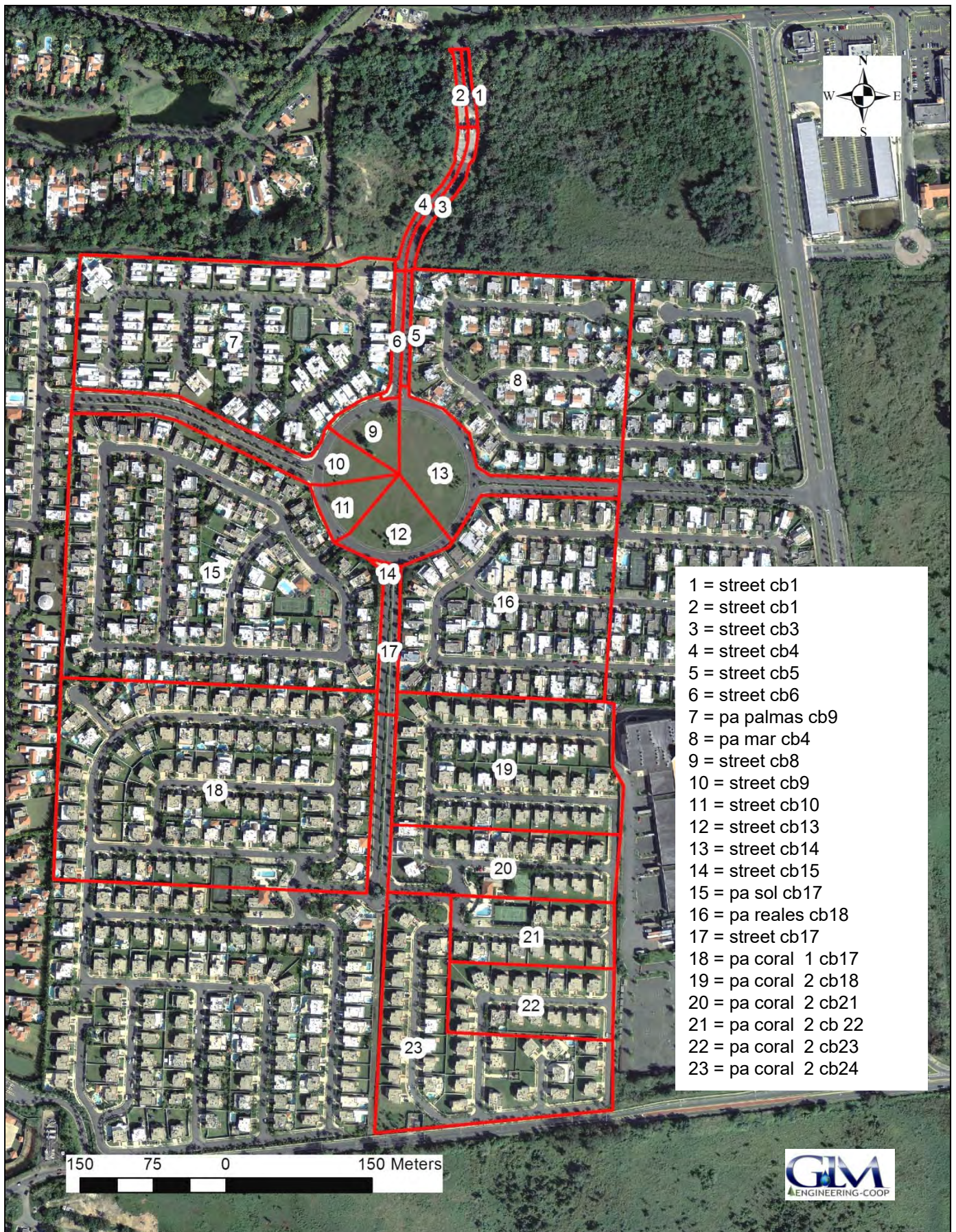
Figure 18: Drainage areas discharging into existing storm sewer
