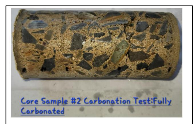
pH Test Result at 0" = 9.7 pH Test Result at 1" = 8.6
