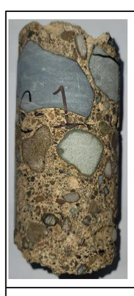
Very porous specimen Bluish gray coarse aggregate 1/16" Plaster
