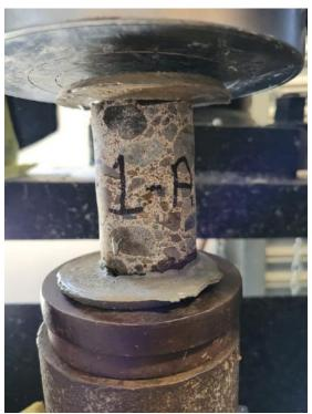
Photo 37: Core sample F-1A before compression test.
