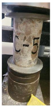
Photo 35: Core sample #5 before compression test.
