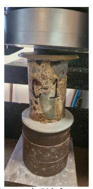
Photo 25: Core sample #1 before compression test.
