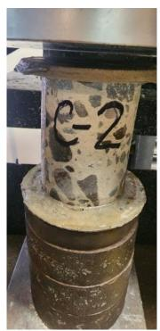
Photo 27: Core sample #2 before compression test.
