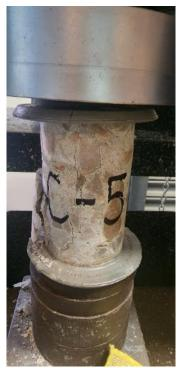
Photo 36: Core sample #5 after compression test.
