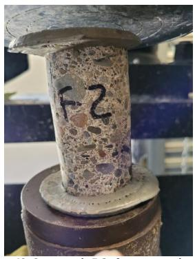
Photo 40: Core sample F-2 after compression test.
