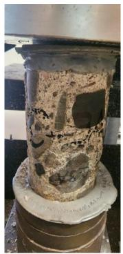
Photo 30: Core sample #3A after compression test.
