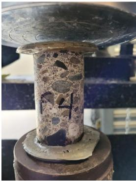
Photo 43: Core sample F-4 before compression test.
