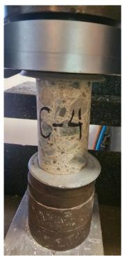
Photo 33: Core sample #4 before compression test.
