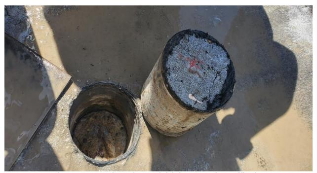
Photo 8: Core performed on roof slab for connection verification.
