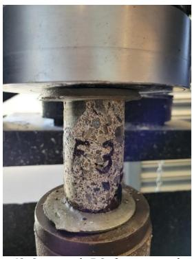
Photo 42: Core sample F-3 after compression test.
