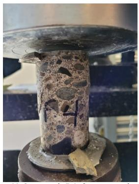
Photo 44: Core sample F-4 after compression test.
