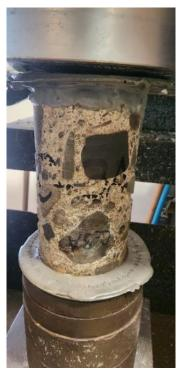
Photo 29: Core sample #3A before compression test.
