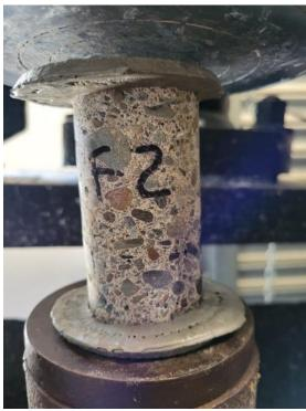
Photo 39: Core sample F-2 before compression test.
