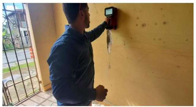
Photo 1: Performing scanning on walls to determine reinforcement layout.
