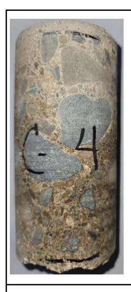
Slightly porous specimen Bluish gray coarse aggregate
