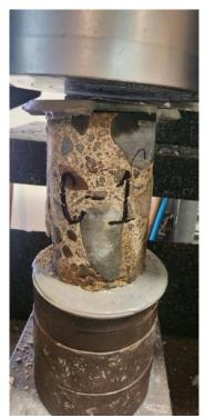
Photo 26: Core sample #1 after compression test.
