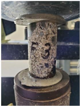
Photo 41: Core sample F-3 before compression test.
