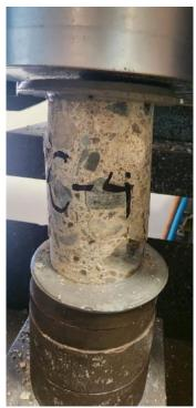
Photo 34: Core sample #4 after compression test.
