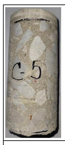
Moderate porous specimen Limestone coarse aggregate ½" plaster
