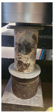
Photo 31: Core sample #3B before compression test.
