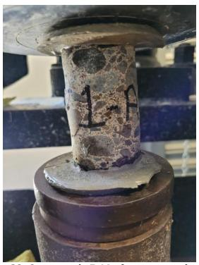
Photo 38: Core sample F-1A after compression test.
