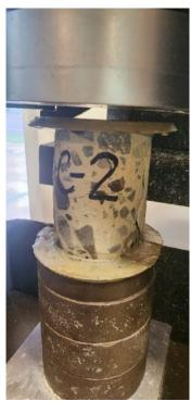
Photo 28: Core sample #2 after compression test.
