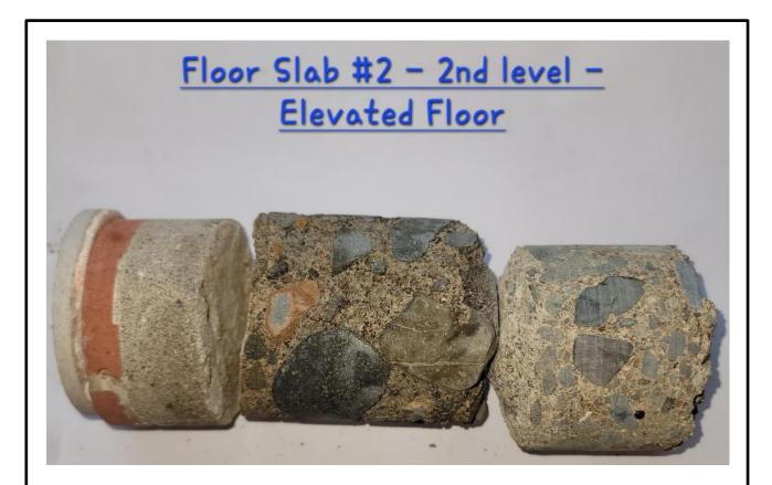
2" Topping and Tile 3-1/2" Concrete Slab 3" Concrete Slab
