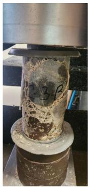
Photo 32: Core sample #3B after compression test.
