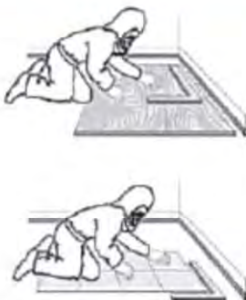
FIGURE 12.10 Install underlayment and new flooring as a suitable LBP enclosure method. The personal protective equipment is for a high-dust project.
