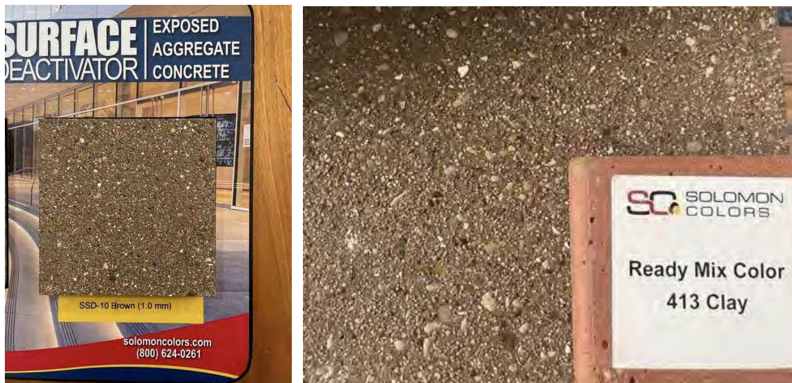
Figure 2. Sample of cementitious material to be applied on the existing concrete slab. Brand: Solomon Colors/Surface deactivator/Exposed Aggregate Concrete; Distributor: Álvarez Trading.)
