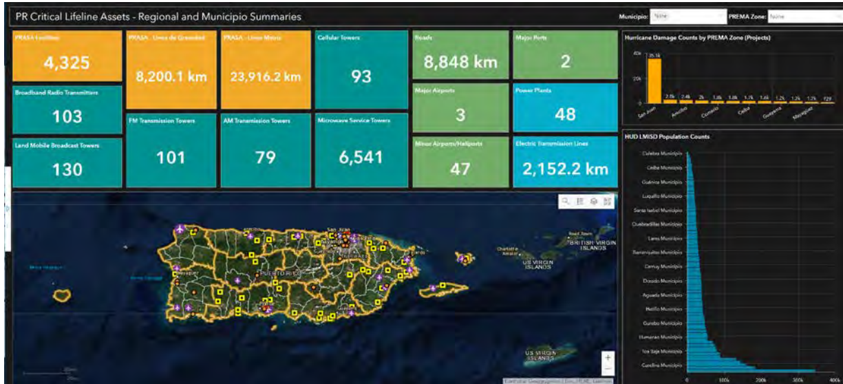
Figure 43. Image of Regional Dashboard depicting geolocation of critical lifeline infrastructure.
