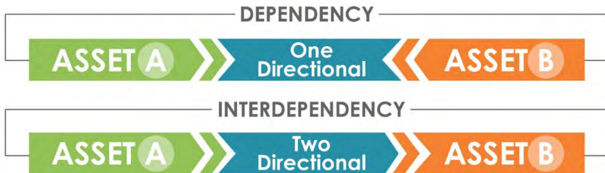
Figure 51. Illustration of definitions for dependence and interdependence. Source: DHS Infrastructure Interdependency Report, Puerto Rico, 2018
